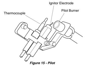
7. Keep control knob pressed in for 10 seconds after lighting pilot. After 10 seconds, release control knob.
